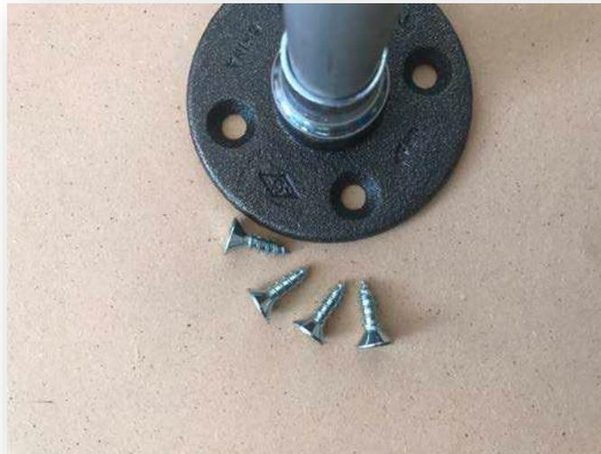
2. Screw in one steel set screw connector into the flange.
