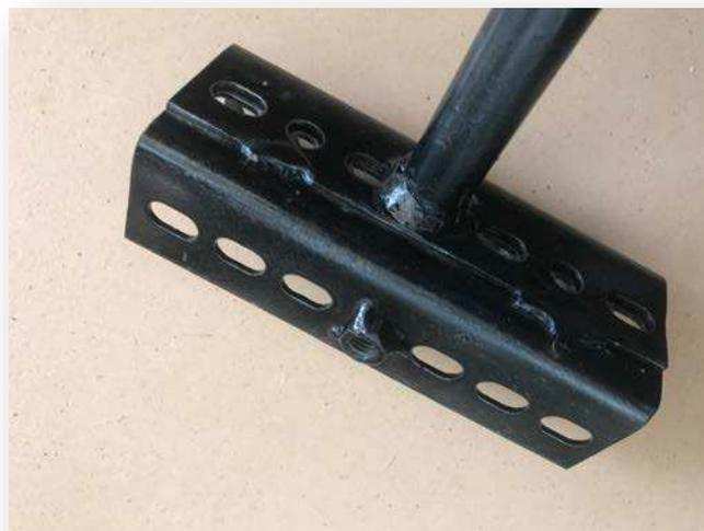
4. Finish by spray-painting the entire clamp frame and tube to avoid rusting. Image shows finished frame and conduit tube.
