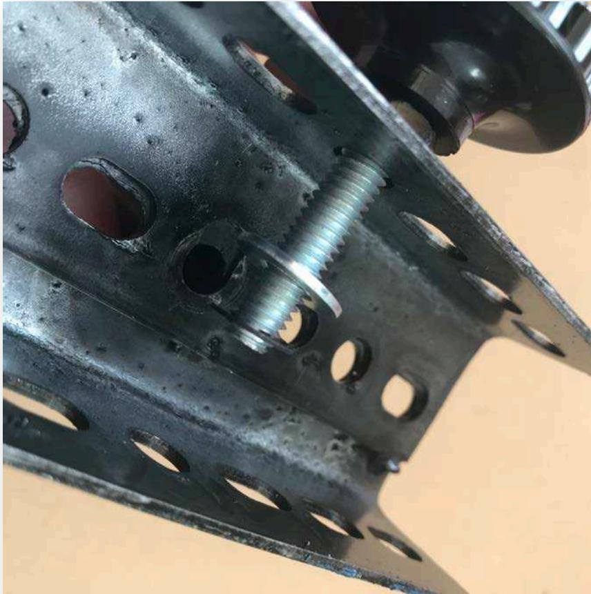
4. Mix up a small amount of epoxy and add a TINY amount onto the last thread of the bolt to
