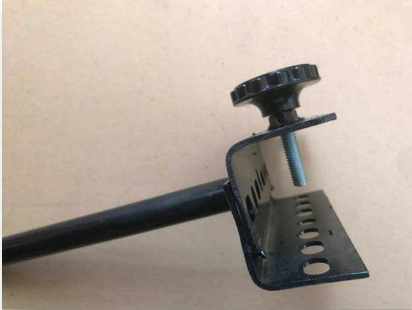
1. Thread the clamping knob through the top hex nut into the center of the clamp frame.
