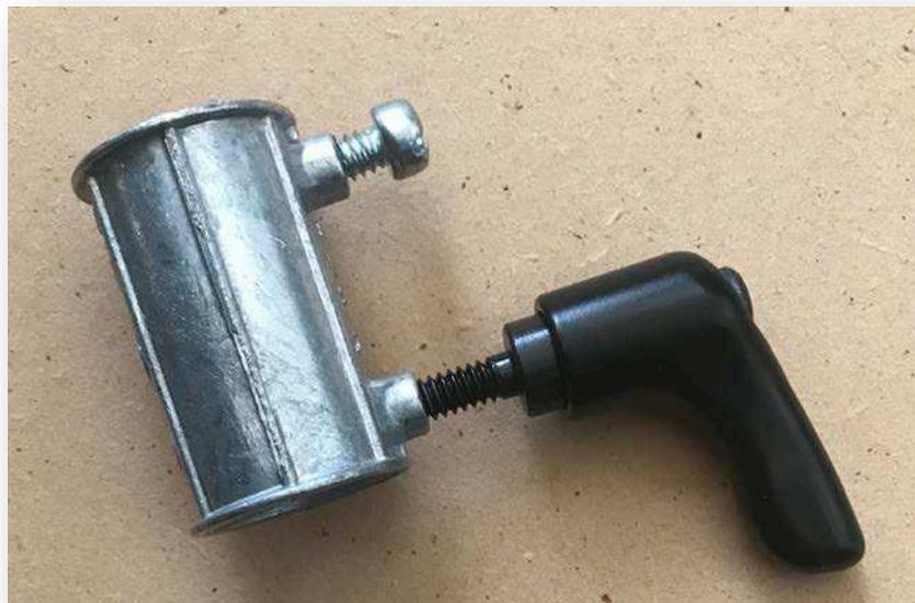
5. Add the above steel setscrew coupler to the top of the 2'6" Emt Conduit tube with the lever positioned as the top set screw. Tighten the bottom set screw in place.
